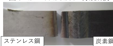
図9. SM490-SUS821L1材破断後
